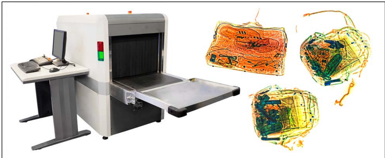
Figure 9-2 Example of an X-Ray Baggage Screening System
